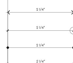
CONCRETE, OR CENTERLINE OF STEEL DIMENSION FROM FACE OF TO FACE OF FINISH DIMENSION FROM FACE OF STUD, CONCRETE, OR CENTERLINE OF STEEL TO FACE OF FINISH [CIRCLED END] DIMENSION END TO END OF CASEWORK
